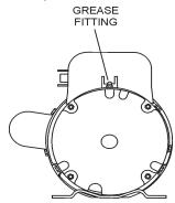
Figure 28. Grease Fittings Electric Motor
